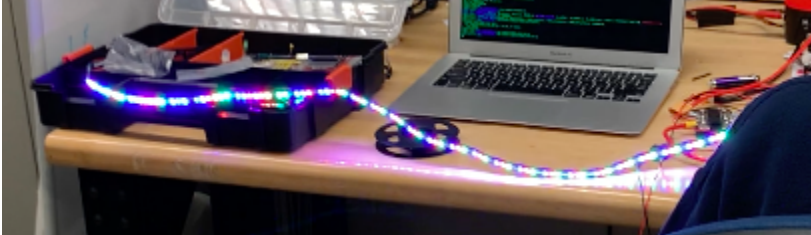
Figure 1. Example of the LED Strip, illuminated using command from Raspberry Pi
